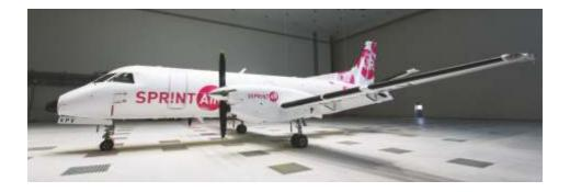
The process of paint application and drying is monitored with the use of hythergraphs recording conditions of painting and drying round-the-clock in the form of records of temperature and relative humidity.
